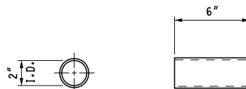
CABLE SLEEVE (FOR POST 1)
